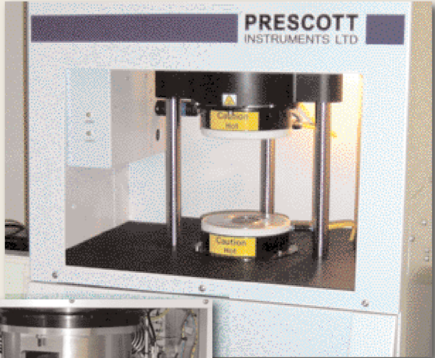
Prescott Instruments' Rheo-Line multi-function rheometer (above) is used to test rubber and elastomer materials. It is based on a frameless and brushless torque motor (left) with a high-resolution optical encoder and integrated servo drive and motion controller
