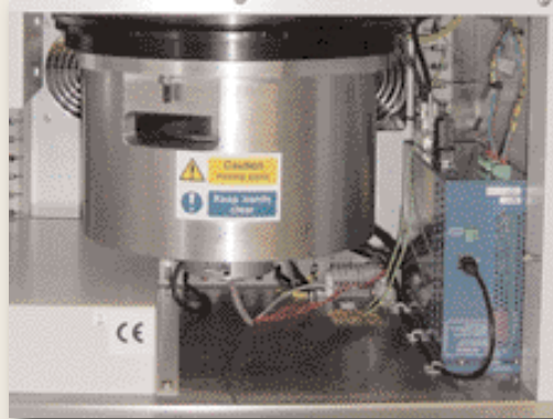
Prescott Instruments' Rheo-Line multi-function rheometer (above) is used to test rubber and elastomer materials. It is based on a frameless and brushless torque motor (left) with a high-resolution optical encoder and integrated servo drive and motion controller
