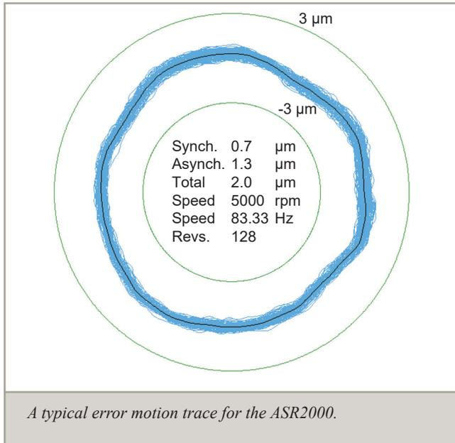
*A typical error motion trace for the ASR2000.*
