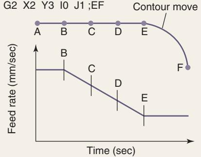
CNC program lines are contained in blocks of G code for describing contouring moves. The controller can look ahead one or more blocks to adjust the acceleration and velocity and ensure the most accurate move for a stage.
