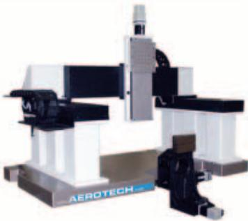
*5-axis precision laser cutting & welding station*
