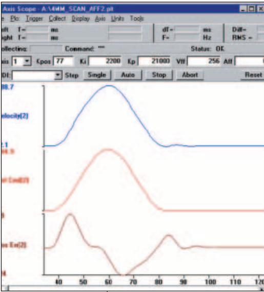
Point-to-point motion and multi-axis contouring moves require high acceleration and bandwidth capability. Move and settle plots such as these can be used to calibrate and monitor positioning accuracy.
