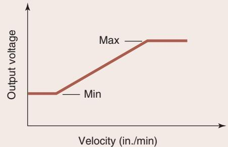
Laser power output is linked to the axes of motion to control the cut kerf and weld width. This technique is called Position Synchronized Output, PSO.
