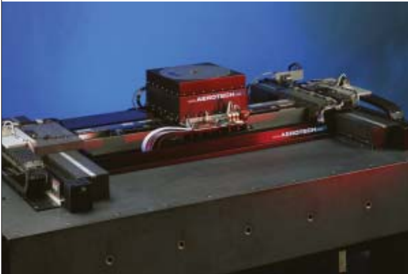
The ABL9000 stage uses air bearings, noncontact linear motors and noncontact optical encoders to provide precise, repeatable X-Y motion without the introduction of wear-induced inaccuracy.
