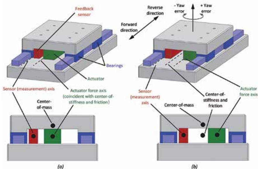
Figure 4. Stage with the actuator placed on the center-of-stiffness and center-of-friction (a) and away from the center-of-stiffness and center-of-friction (b).
