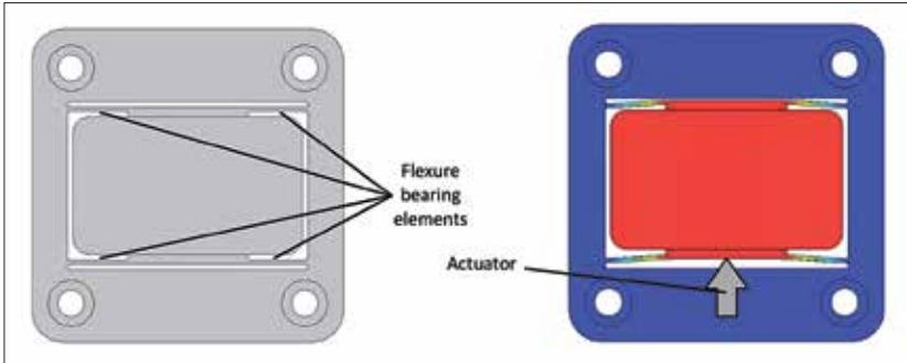
Figure 1: A flexure bearing, when actuated flexes (deforms), causing motion of a positioning system component.
