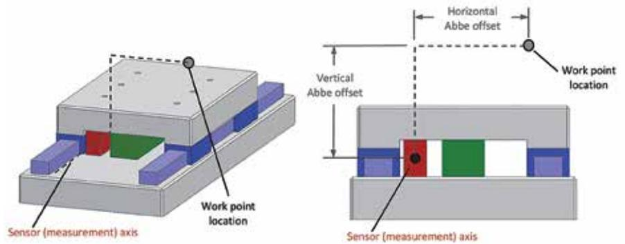
Figure 5. It is best to place the sensor at the process point of interest, due to the effect of Abbe error.
